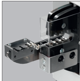
Detail Schutzhaube/ detail protection cover
